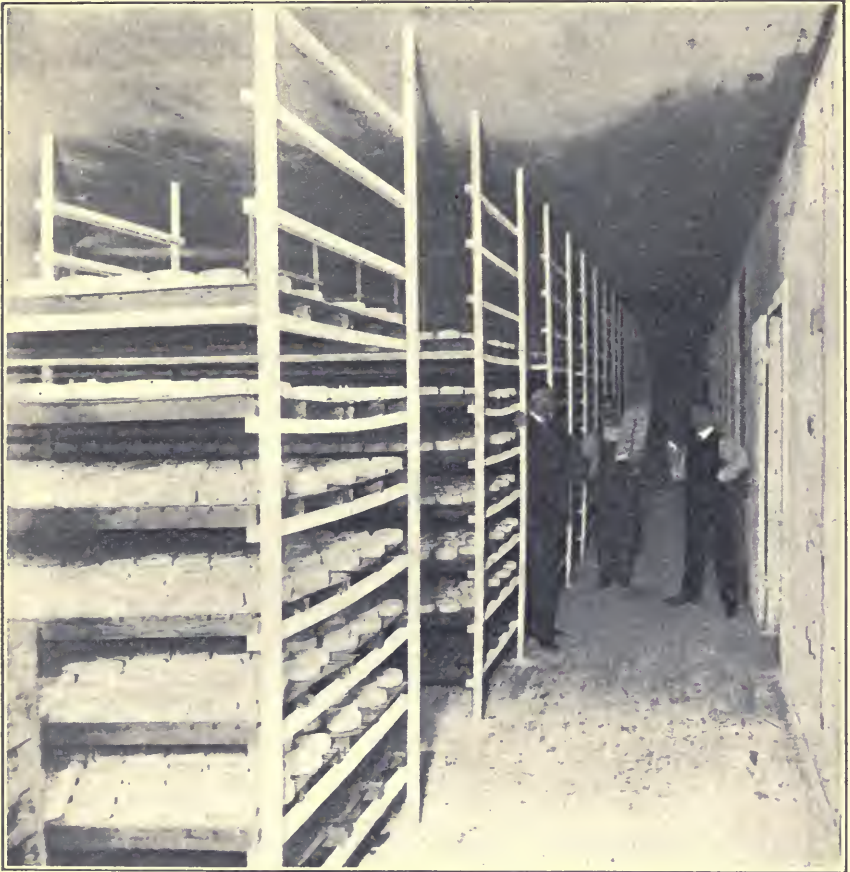
FIG. 3.—“Halloor” or first ripening room in American Camembert factory, showing arrangement of shelves and cheeses upon them.
