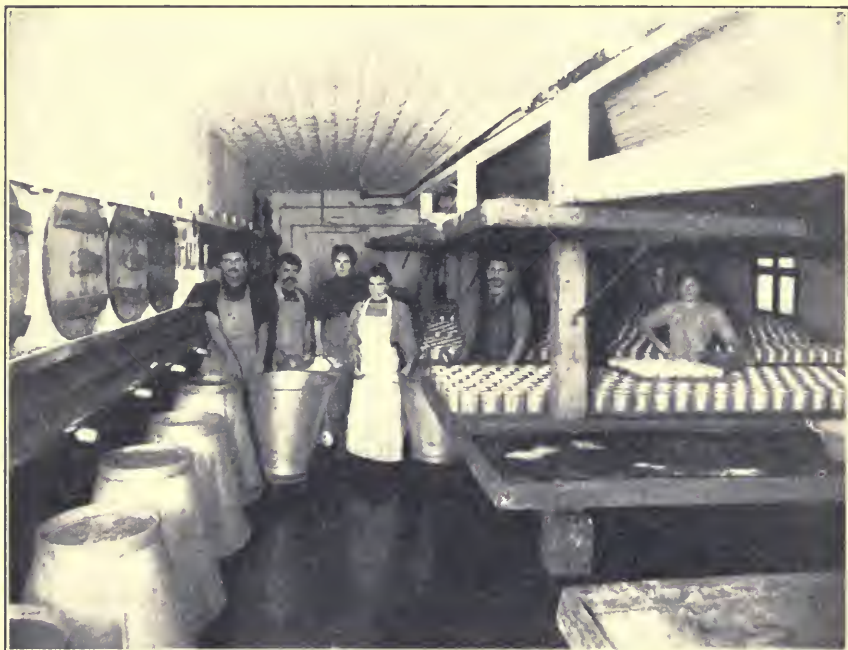
FIG. 1.—Camembert cheesemaking room in American factory, showing arrangement of tables, aisles, curdling cans, and milk-distributing pipes.
