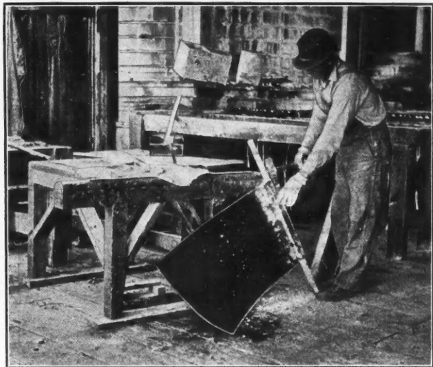
CUTTING OUT CONDUCTOR BARS FROM SPENT ANODES
