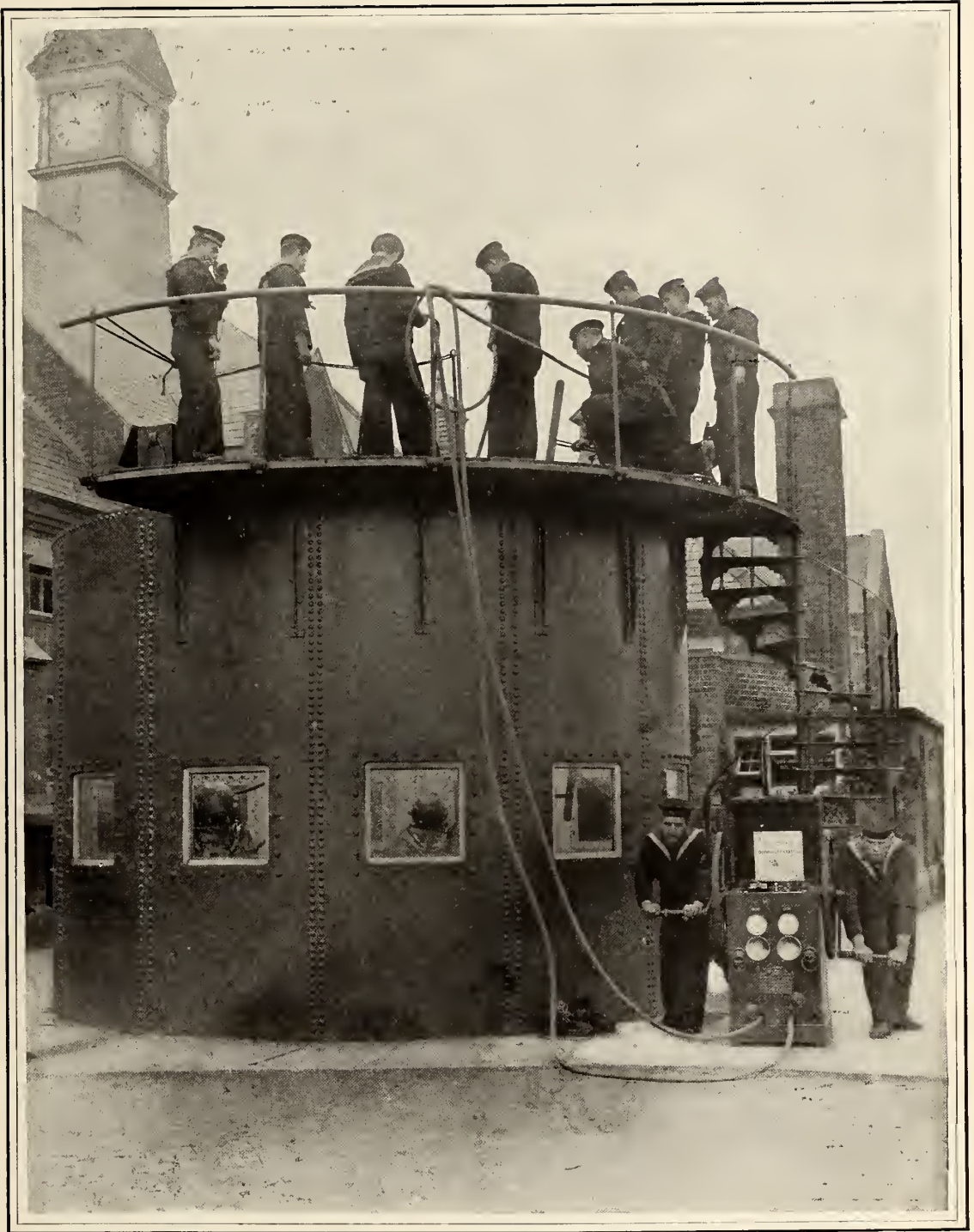
THE LARGE DIVING TANK FOR GIVING PRACTICE TO NAVAL DIVERS. THROUGH THE SQUARE WINDOWS CAN BE SEEN TWO OR THREE IN DIVING-SUITS IN THE "WATER-SCHOOL."
