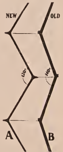
Drawing illustrating the difference between the Airoo foundation A, and the old foundation, B. The latter has the thicker base, the flatter angle, and the unavoidable distortion.
