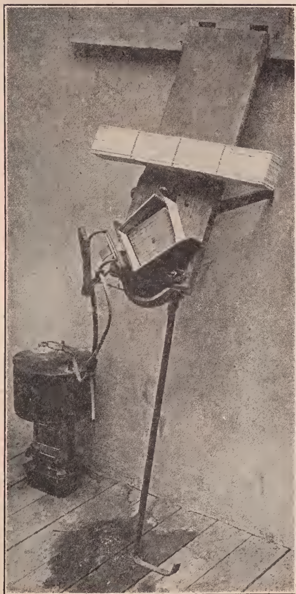
The Root section-folder and steam foundation-fastener. Steam is generated in the small boiler, rises thru the tube and keeps the plate at a constant and uniform temperature.
