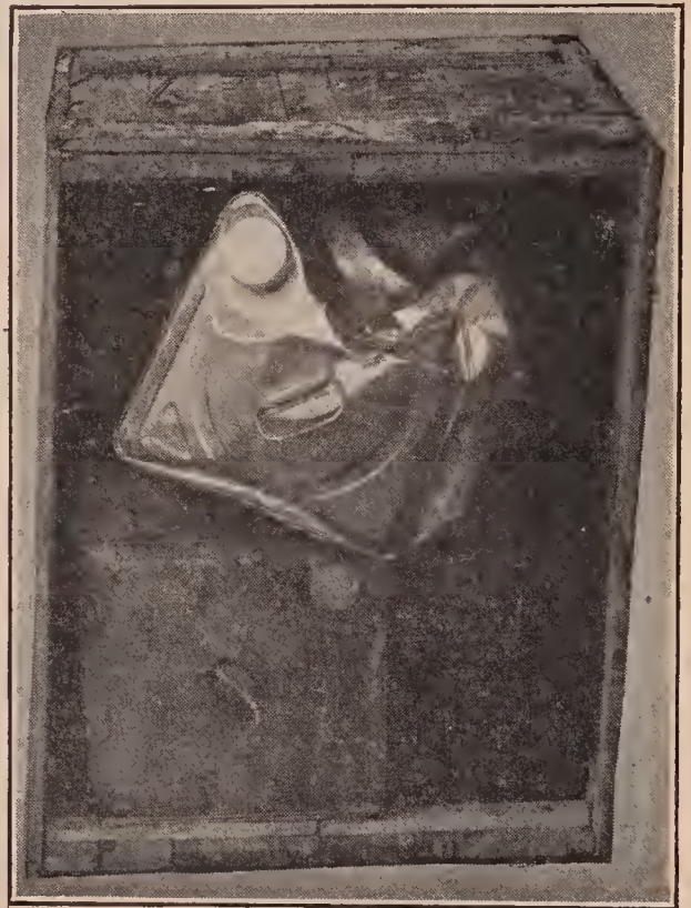
A honey can after being shipped loose in a box. Most of the honey had leaked out.
