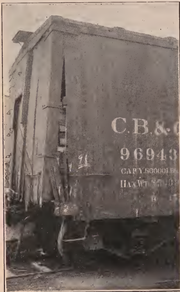
Why honey needs solid bracing in a car. In this instance the car was bumped so violently that the honey went right on thru the end.
