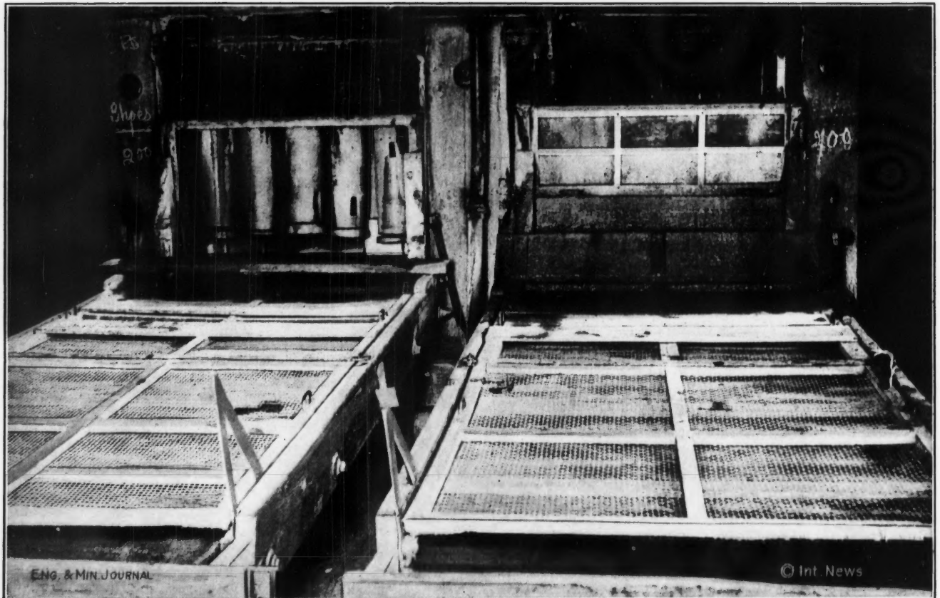
TRANSVAAL STAMPS WITH LOCKED GUARDS OVER PLATES TO PREVENT THEFT OF AMALGAM
