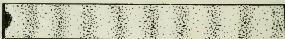
FIG. 1. DIAGRAM OF A SOUND WAVE IN AIR. Wave-length, one centimeter. Wave-time, 0.3 ten-thousandths of a second.
