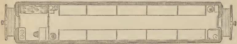
FIG. 6.—Horizontal plan of one of the hospital cars of the Army of the Potomac.—(OTIS.)
