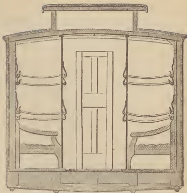
FIG 8.—Transverse section of one of the hospital cars of the Army of the Potomac.—(OTIS.)
