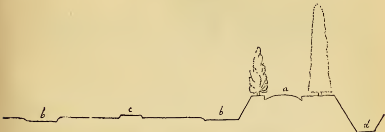
Fig. 82. Section across the Terrace, and one of the Double Beds for Graves.
