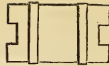
Fig. 42. Elevation of the End C in fig. 38., which is 2 in. shorter than the End B.
