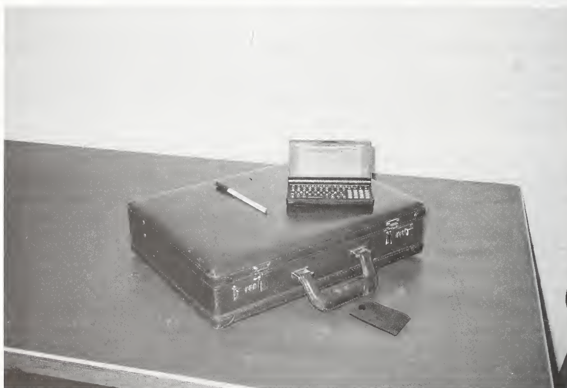
Photograph of Prototype ITMS (Hand-held transit information computer)
