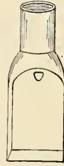
FIG. 33.—A badly-shaped self-cleaning drill. Shoulder does not fill the hole, and drillings rush past the opening without lifting valve with maximum force. This is, however, a very good shape for a jetting outfit.
