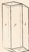
Fig. 12a. Hornblende. Prisma p = \{110\}, \infty P ; Klinopinakoid b = \{010\}, \infty P\infty ; Basis c = \{001\}, oP ; Positive Pyramide o = \{11\bar{1}\}, + P .
