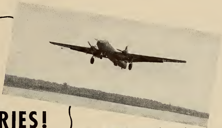
NAVY'S NEWEST reconnaissance plane, the Martin XP4M-1 has 4 engines, tandem-mounted in 2 nacelles. Two reciprocating engines, two jet, provide fighter plane speeds when needed.
