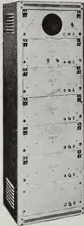
(Left) "12000 SERIES," 80 Watt Amplifier—built on the easy unit-service and replacement basis—utilizing four 20 watt power amplifiers—wired to enable projectionist to use 20—40—60 or the full 80 watts as needed. Built-in, self-powered monitor speaker, electronic equalizer panel, separate wide range high and low frequency response controls.
