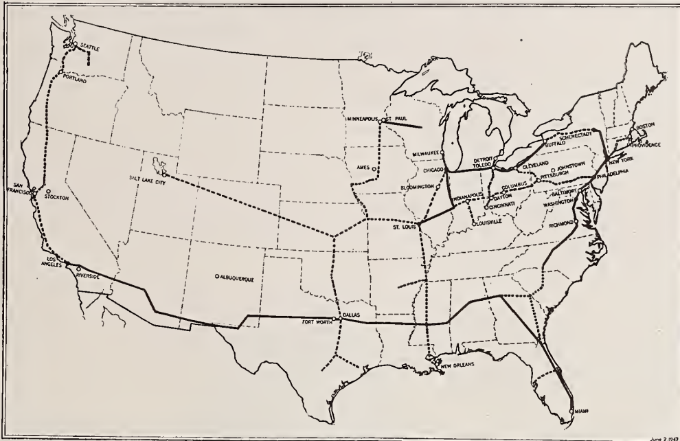
The American Telephone & Telegraph Company coaxial cable network, now in work and partly completed, is shown on this map. The solid lines indicate cables installed or under construction in 1947. The broken lines indicate cable and radio relay extensions planned. Solid dots are television stations now in operation, and the open circles are stations approved by the FCC for construction.
