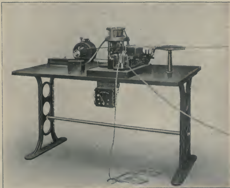
FIG. 2.—Creed type printer (translating from perforated Morse strip).
