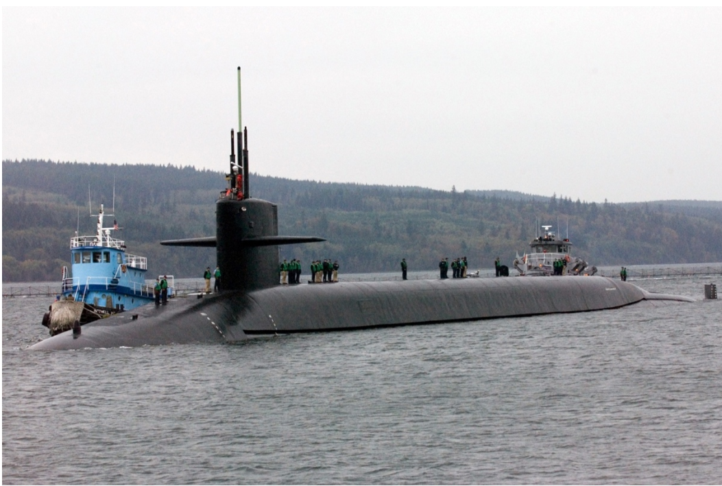
Figure 13: Ballistic Missile Submarine Superstructure ("Turtleback")
