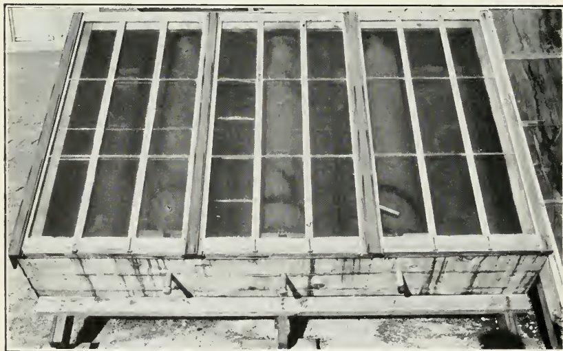
2. TRIPLE-TANK ABSORBER IN INSULATED BOX WITH HOTBED SASH COVER.
