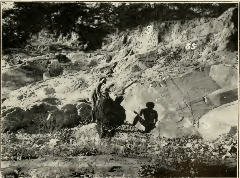
2. OLD QUARRY ALONG TILDEN STREET (NEAR CONNECTICUT AVENUE), ILLUSTRATING WEATHERING OF THE HARD JOINTED GRANITE (G) INTO SUBSOIL (SS) AND THEN SOIL (S).
