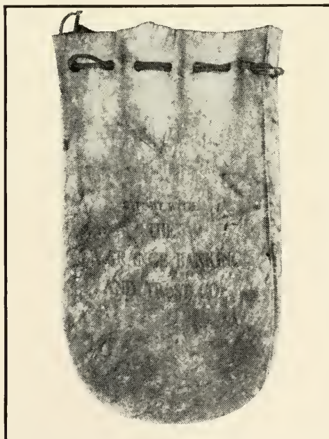
2. SAME MONEY BAG PHOTOGRAPHED WITH INFRARED RADIATION, SHOWING LETTERING THAT PERMITTED THE DECIPHERING OF THE NAME OF THE BANK FROM WHICH IT CAME.
