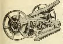
THE IMPERIAL is one of our best Mowers, the principal feature being that the knife is securely bolted to the sides, thus insuring a perfectly rigid frame. The knives are adjusted by means of our patent hanger, and a locking screw holds them sesurely in place. This hanger is so constructed that all wear can
