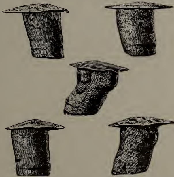
SOME DEFECTIVE RIVETS.
