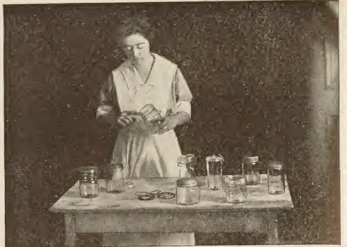
FLAWS IN THE GLASS WHICH INTERFERE WITH THE SEAL MAY BE DETECTED BY RUNNING THE FOREFINGER AROUND THE RIM OF THE JAR
