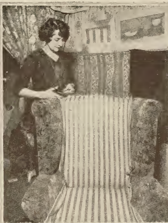
TO CUT THE MATERIAL, LAY THE BACK LENGTH OVER THE CHAIR. BE SURE THE MATERIAL IS STRAIGHT
