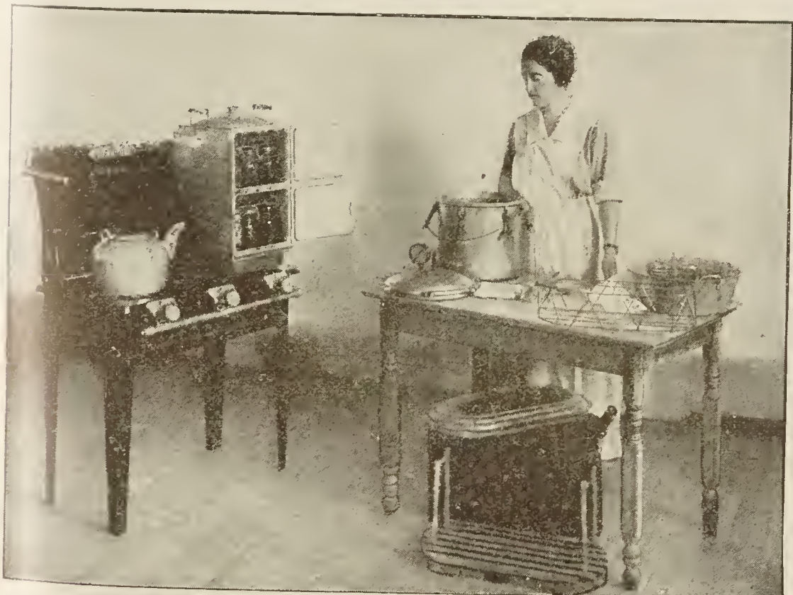
CANNING EQUIPMENT FOR HOME USE; THE HOT-WATER OUTFIT, CONSISTING OF A WASH-BOILER AND A RACK; OR THE STEAM COOKER; AND THE STEAM-PRESSURE COOKER
