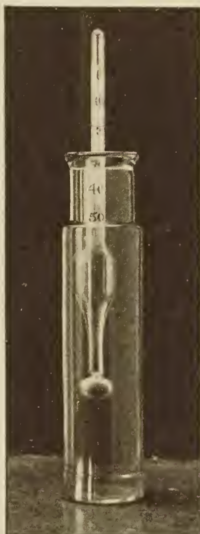
A SACCHAROMETER MEASURES THE THICKNESS OF THE SIRUP
