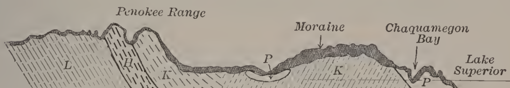
FIG. 3.—The north end of the cross-section mentioned under Fig. 2. Strata much disturbed from their horizontal positions. L , Laurentian (granite group); H , Huronian (granite group); K , Keweenawen (copper-bearing group); P , Potsdam sandstone. The surface-rock of the cross-section between Figs. 2 and 3 is Laurentian granite.
