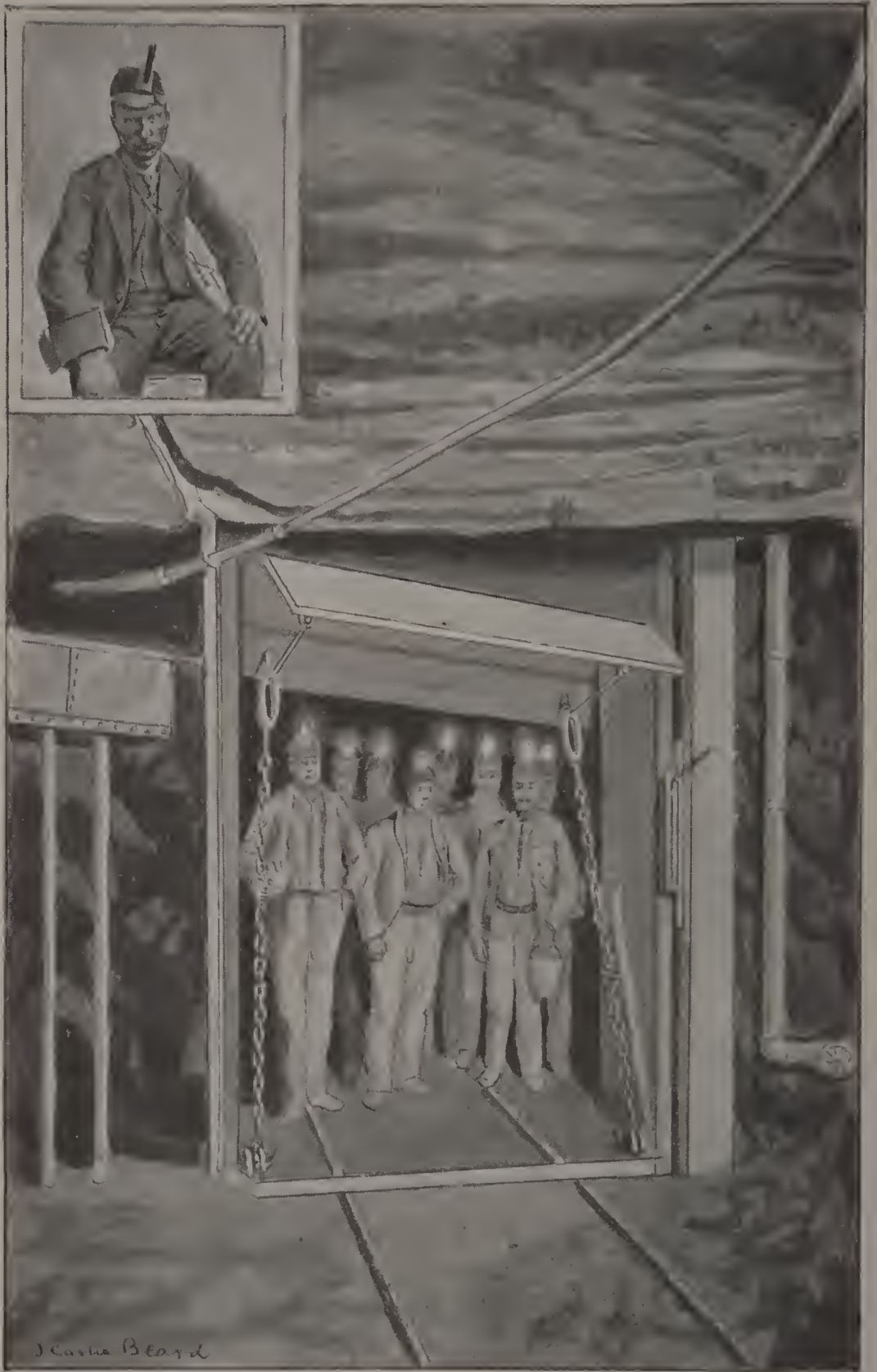
FIG. 29.—Coal-mine, showing miners in cage at the bottom of the shaft. Part of mine and tramways on which the small cars are pushed to the shaft.
