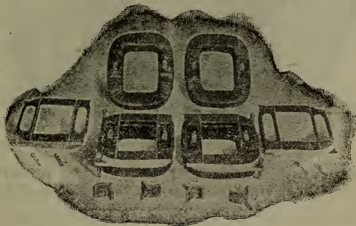
FIG. 81. GENERATOR FIELD COILS AND RETAINERS.
