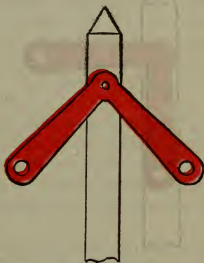
FIG. 107. A RIGHT-ANGLE SEMAPHORE FOR BLOCK SIGNALS WHEN USED ON A DOUBLE TRACK, FOR TRAIN-ORDER SIGNALS ON SINGLE TRACK.
