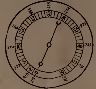
TEMPERATURE OF STEAM FROM ATMOSPHERIC TO 50 LBS. PRESSURE
