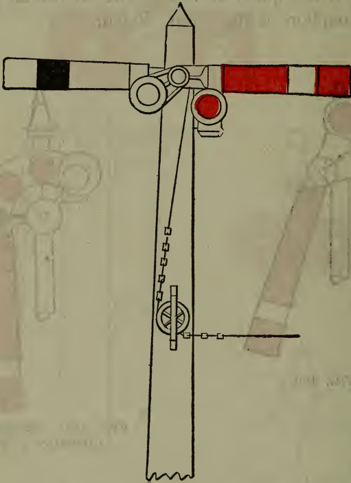
FIG. 102. A TWO-POSITION TRAIN-ORDER SIGNAL.
