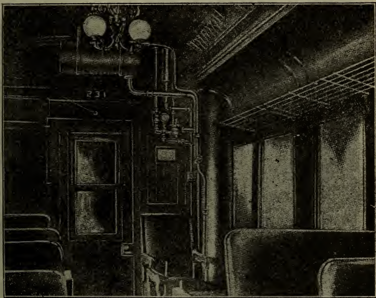
FIG. 59. INTERIOR OF COACH, WITH GAS GENERATOR INSTALLED.
