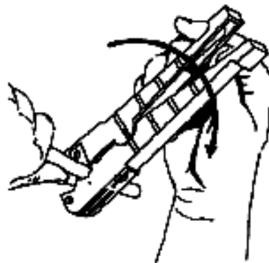
Figure 13. Coaxial Cable Stripping
