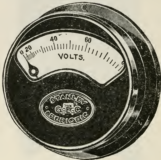
No. 17.—G.E.C. Volt Meter.
