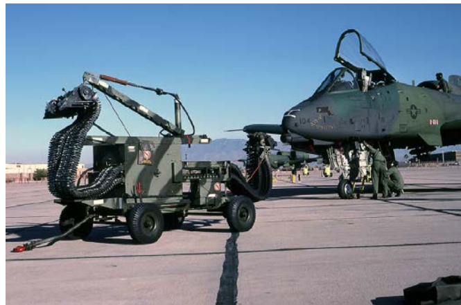
Figure 20. GAU-8 ALS, required for A-10 gun reloads 138
