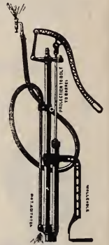
Fig. 632. Myers Lever Bucket Spray Pump
