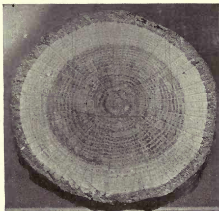
FIG. 179. — Cross section through the stem of a Red Oak, showing heartwood and sapwood.
