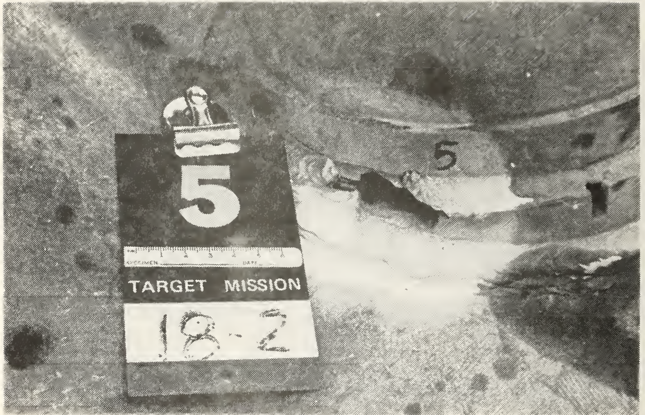
Fig 14. Close-up View of Perforation Through Loader's Periscope Housing, Mission 2, Target 18
