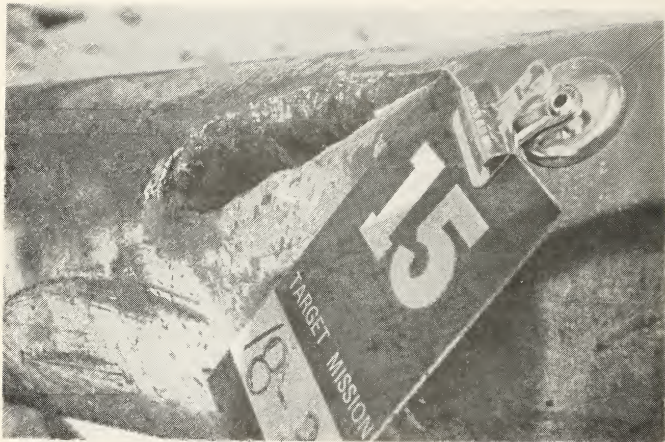
Fig 29. Penetrated Wall of Gun Tube Impact 15, Mission 3, Target 18
