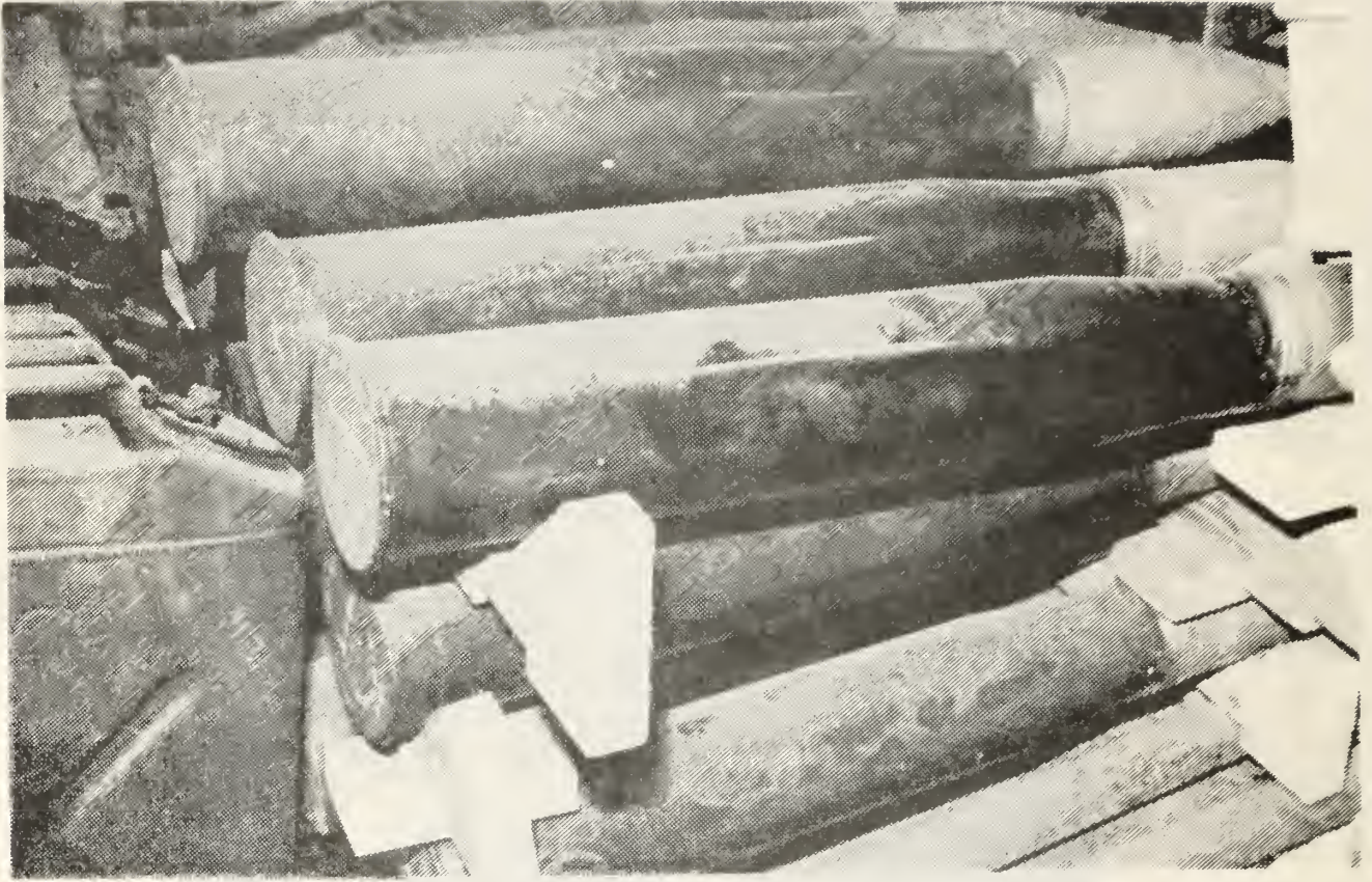
Fig 4. Simulated Fuel Tank and Rear Fighting Compartment Ammunition Stowage
