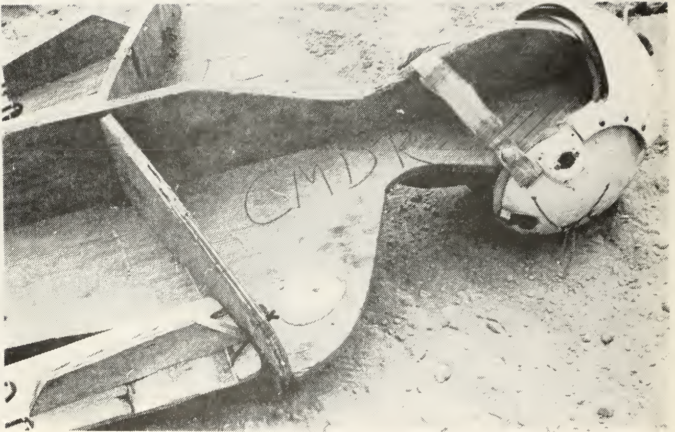
Fig 16. Projectile and/or Spall Damage to Mannikin at Commander's Station (Impact 5, Mission 2, Target 18)
