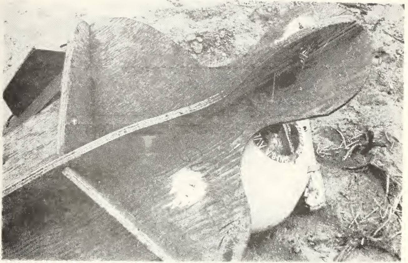
Fig 15. Projectile and/or Spall Damage to Mannikin at Gunner's Station (Impact 5, Mission 2, Target 18)
