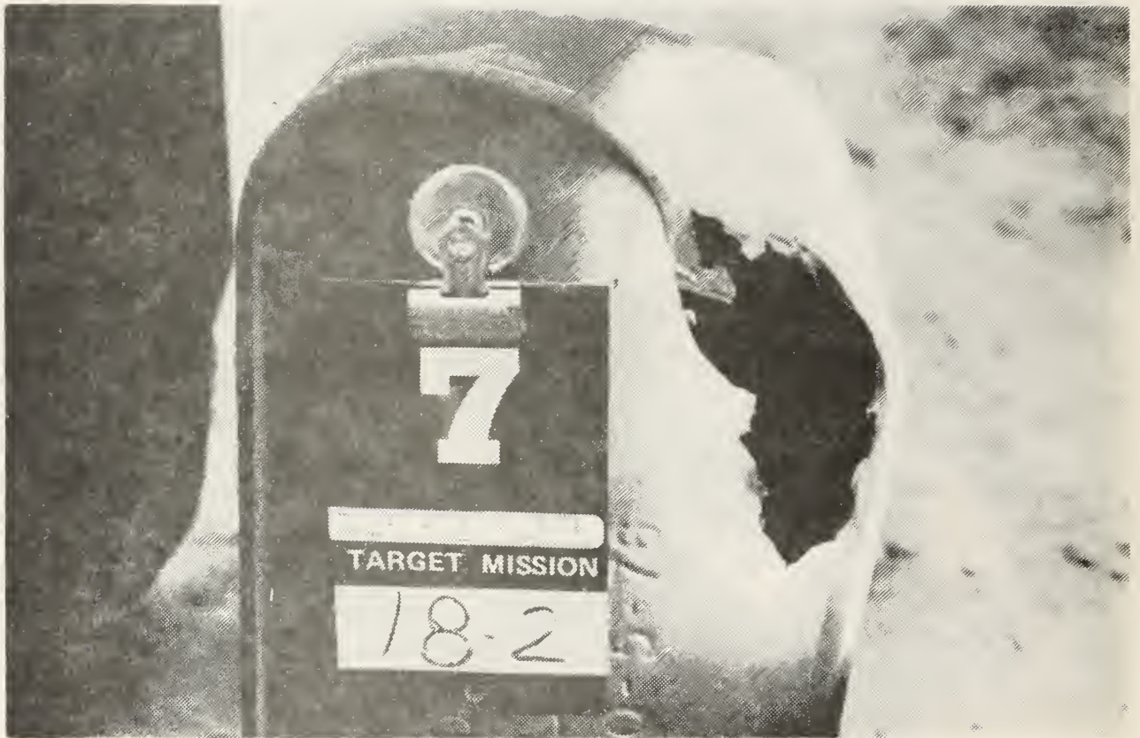
Fig 22. Perforation of Fuel Can Simulating Bow Fuel Tank, Impact 17, Mission 2, Target 18 (NOTE: This impact is mis-numbered and should read 17.)
