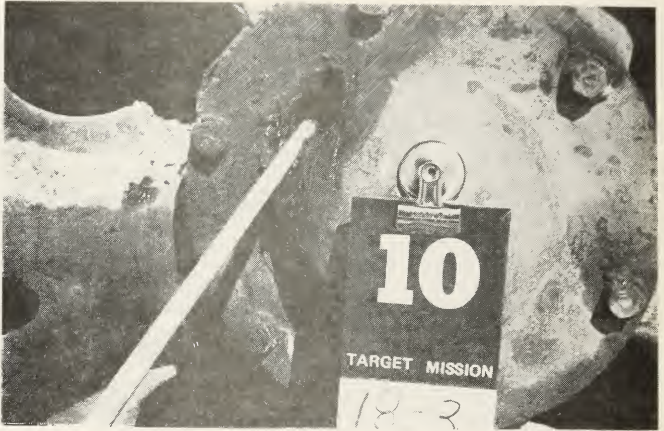
Fig 31. Impact 10, Mission 3, Target 18 Showing Damage to Right No. 1 Road Wheel
