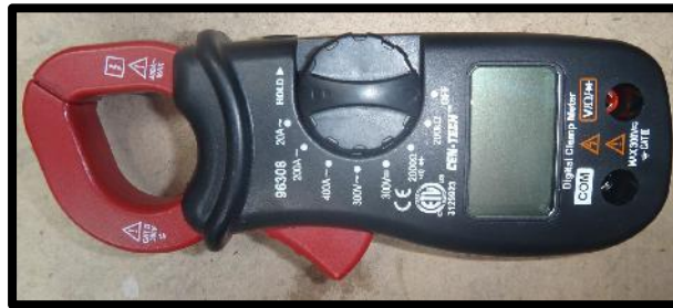
Figure 25. Clip on ammeter used to measure current.
