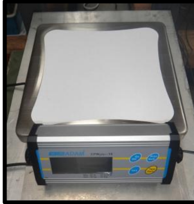
Figure 20. Digital balance used for thrust measurement.
