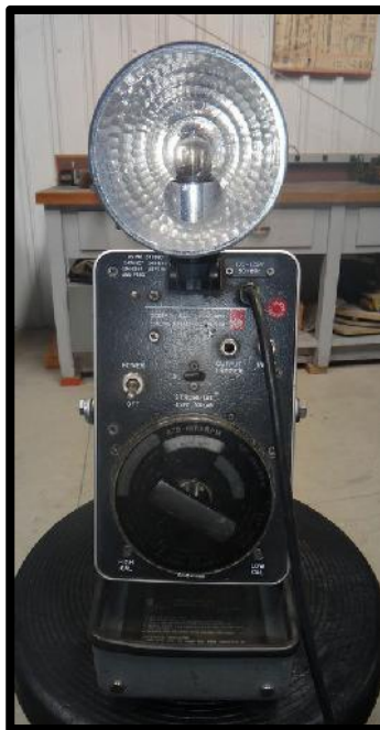
Figure 23. Strobe tachometer used to measure speed.
