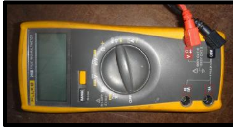
Figure 24. Fluke multimeter used to measure voltage.
