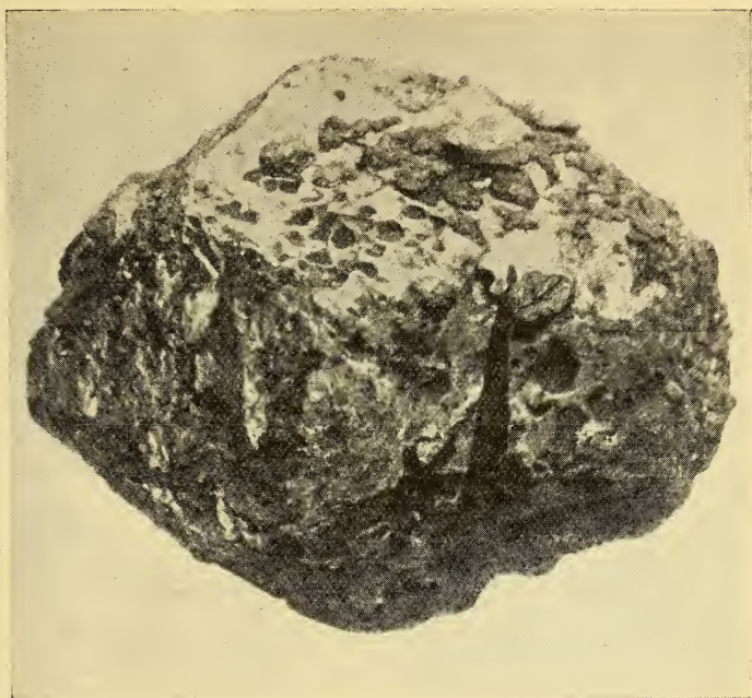
Fig. 3—Crystals of Native Silver seated on a crystal of native copper, Lake Superior. 2 diams.
