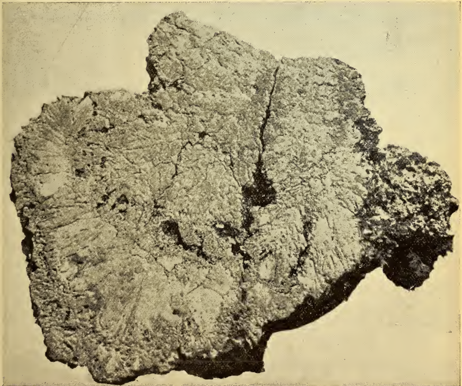
Fig. 6—Section of a nugget of native copper, Burra Burra, South Australia. 2 diams.
