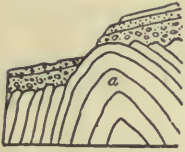
FIG. 1. Anticlinal axis at a . Strata disturbed, folded, and denuded, and afterward unconformable strata deposited upon them, followed by conformable layers.
