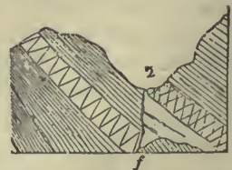
FIG. 4. Strata inclined but conformable. Fault from f to 2 and dyke in the fault.
