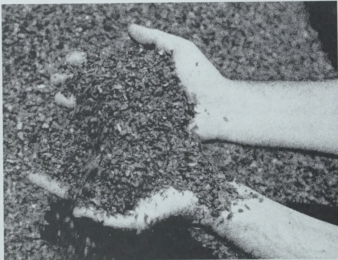
Bark ground to a uniform size, ready for drying
