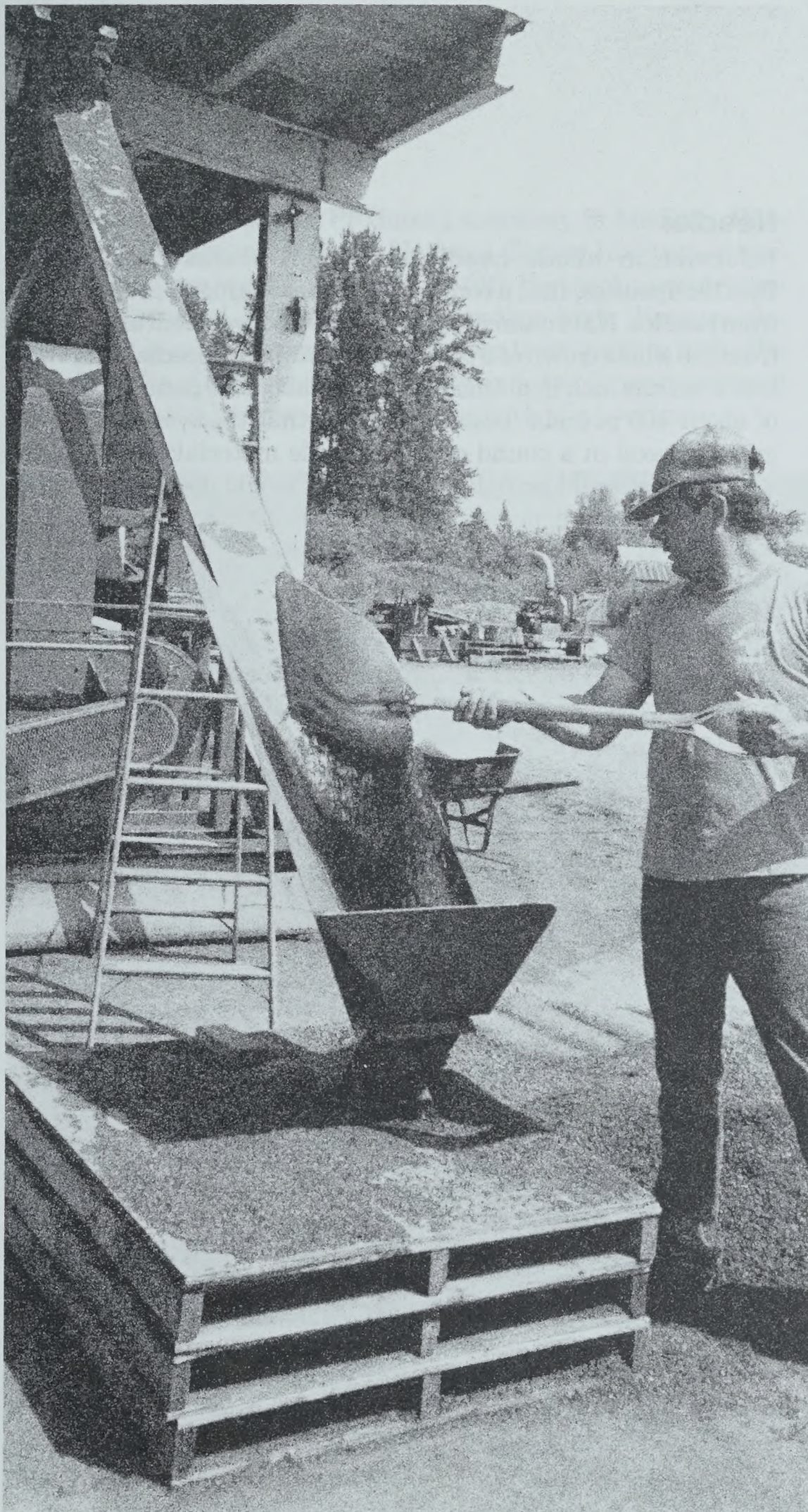
A worker loads ground bark onto a conveyor belt leading to the dryer
