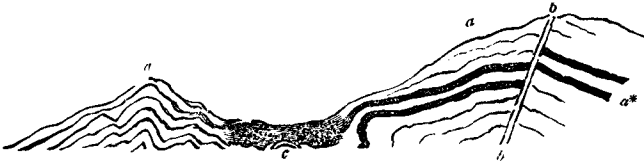
a. Contorted culm strata with stone coal. b. Fault. c. Slash of finely triturerated culm between violently contorted strata, and probably upon a great line of fracture.
