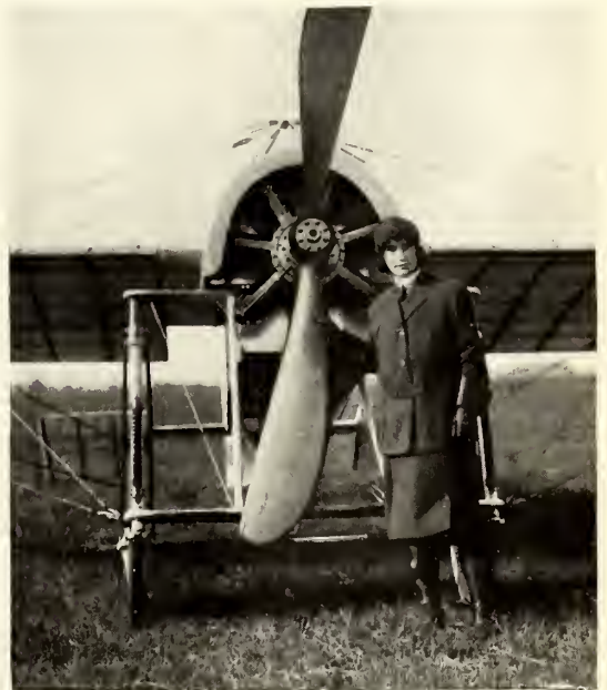
FRONT OF MONOPLANE, SHOWING PROPELLER AND ROTARY ENGINE.
