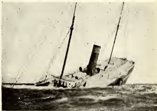
A SHIP THAT FLOATED THREE HOURS AFTER DAMAGE, AND SANK ONLY BECAUSE HER DECKS AND BULKHEADS YIELDED UNDER THE INCREASING PRESSURE OF THE SEA.
