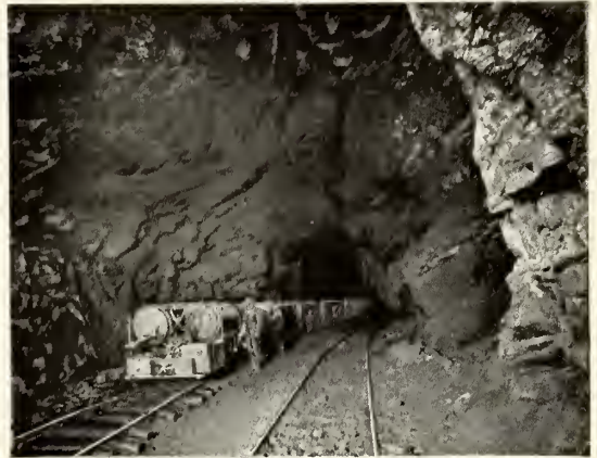
A DOUBLE-CYLINDER COMPRESSED-AIR LOCOMOTIVE IN A UTAH COAL-MINE.
