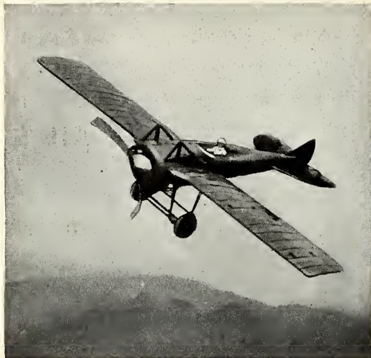
THE DEPERDUSSIN RACING MONOPLANE. IT HAS AVERAGED 125 MILES AN HOUR.
