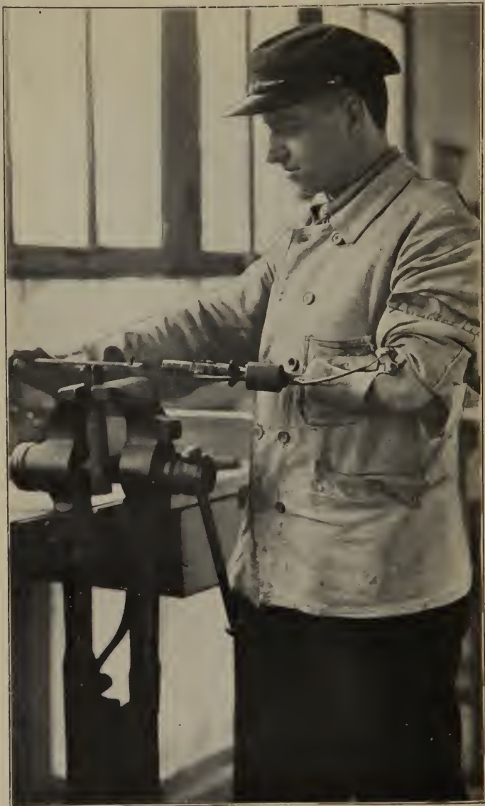
A "Working Arm" in lieu of Nature's Own. A variety of tools can be fitted into the chuck of this appliance, and the one-armed poilu is again enrolled in the army of labor
