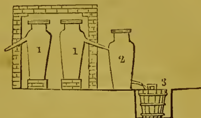
Distillation of Native Sulphur.
