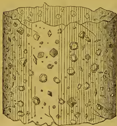
Magnified portion of a Tube lined by the Sublimed Crystals of Arsenious Acid.
