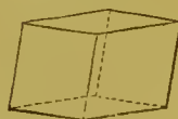
Oblique rhombic prism (principal form of sulphur by fusion and slow cooling).
