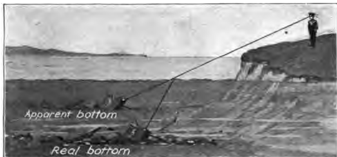
FIG. 27. — Showing why a pool of water looks shallower than it really is in consequence of refraction. The looker-on imagines the bottom to be in a straight line in which he is looking, while in reality it is in the direction of a bent line and lower down.
