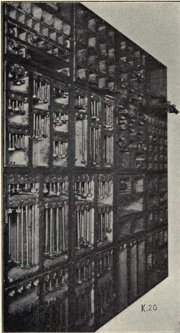
FIG. 87. — Tool-room section made up of tiers of racks, and each compartment subdivided with boxes labeled with brass plates, giving the size and symbol of the bolts contained therein. Particular attention is called to the method of stocking the bolts; the sizes and lengths of the bolts regulate the sizes of the boxes. Pegs are provided on the front of the bottom beveled edge for the workman's checks.
