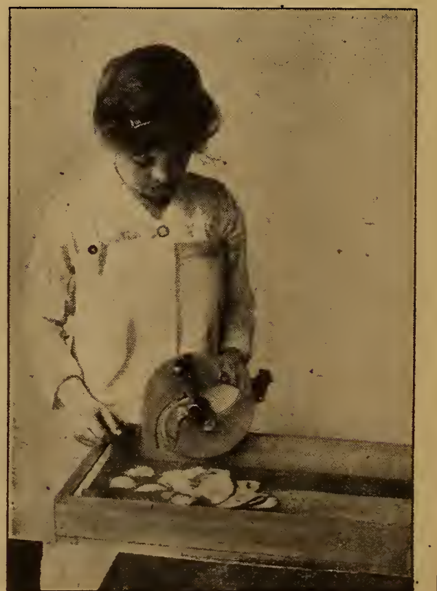
Close view of machine potato slicing, making possible any desired thinness of potato "chips"
