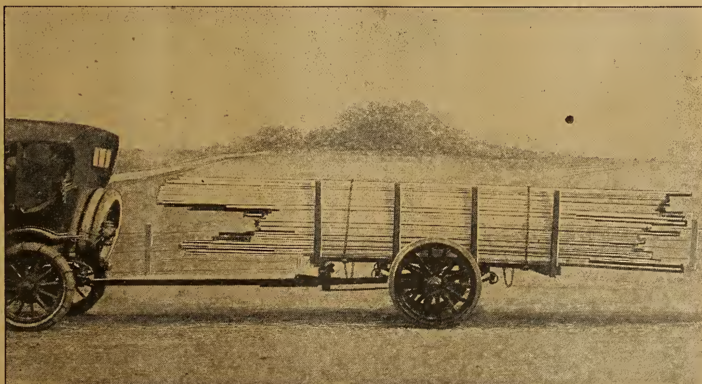
The load on this sturdy trailer is 200 feet of barn siding weighing 3,020 pounds. The automobile pulling it has a 35-horsepower motor. A spring hitch prevents strain when starting and stopping
