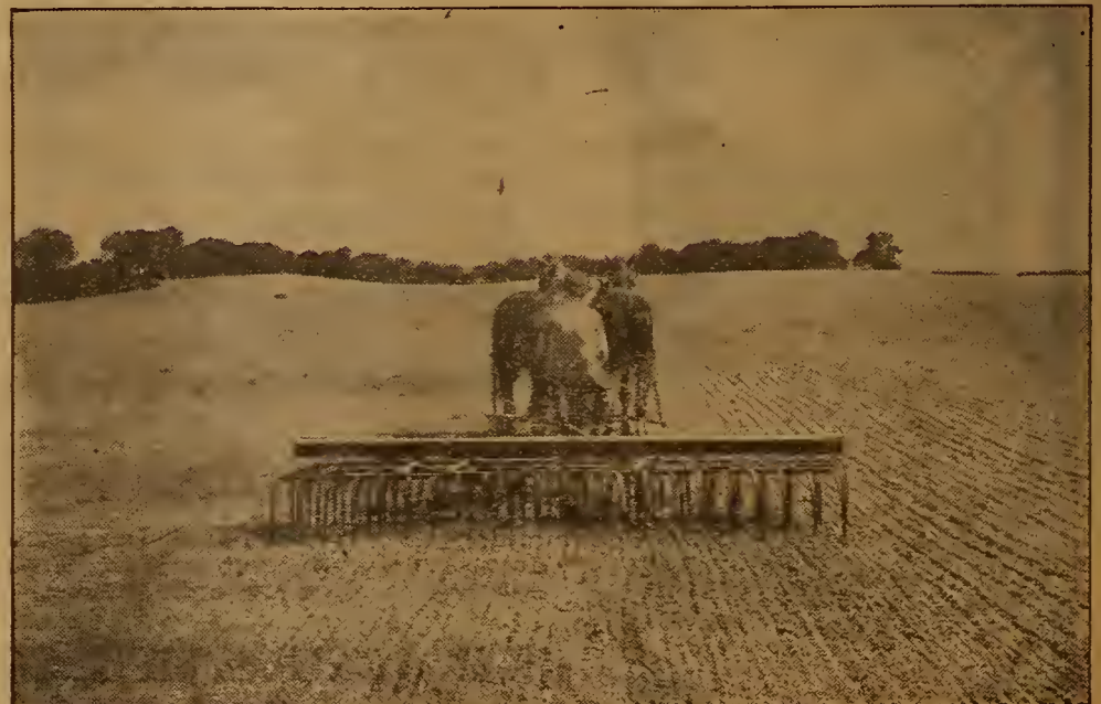
The weeder teeth may be set by means of a lever in front of the driver to cover the seed either shallow or deep
