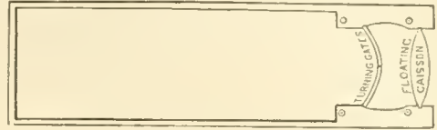
Fig. 2.—Plan of dry dock at Brooklyn navy-yard.
