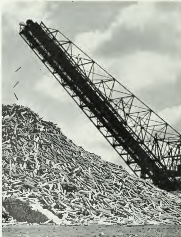
BUILDING PULPWOOD RESERVE PILE AT MILL
