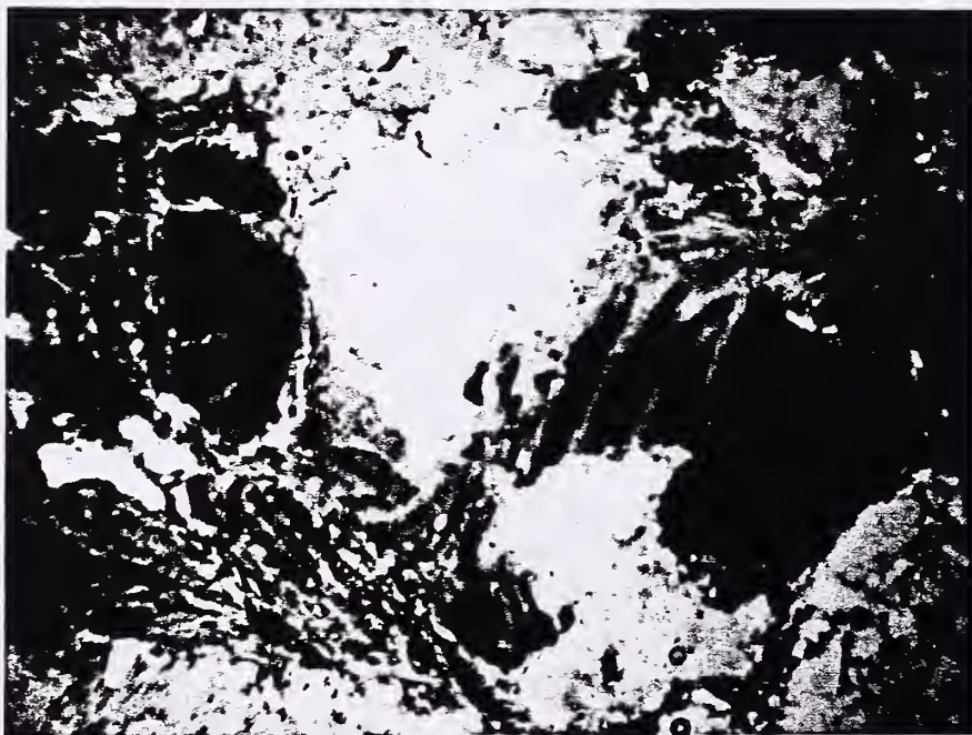
Figure 8.--Weathered biotite grains exhibiting iron oxide staining of adjacent feldspars and partial alteration of biotite to iddingsite and smectite. Magnification = 40X; plane light.
