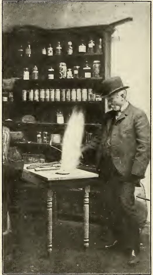
FIG. 13. SETTING FIRE TO SMOKELESS POWDER. THE LIGHT FLARE IS FLAME ONLY, WITH NO SMOKE.
