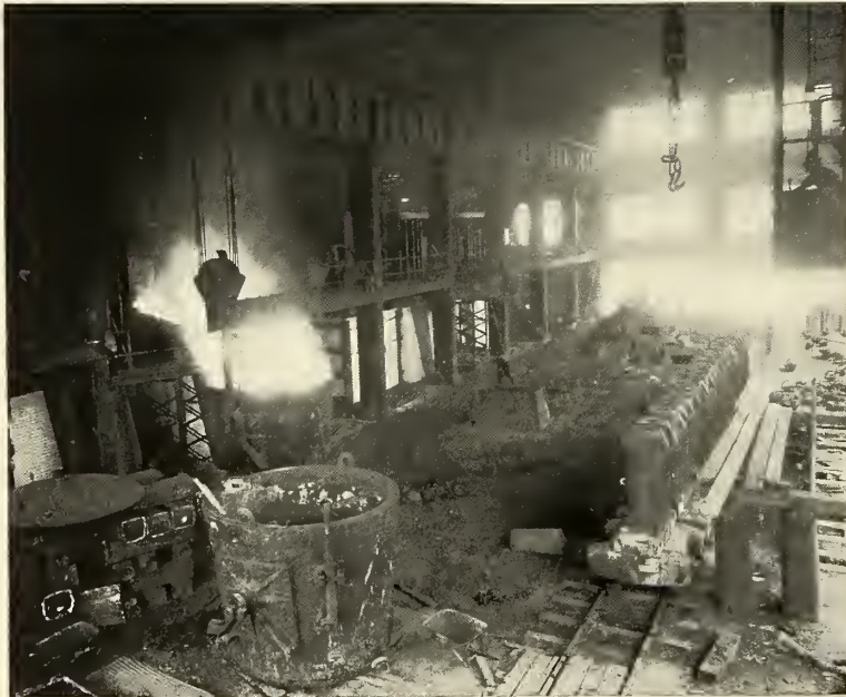
FIG. 13. "POURING" INTO A LADLE FROM AN OPEN-HEARTH FURNACE.
