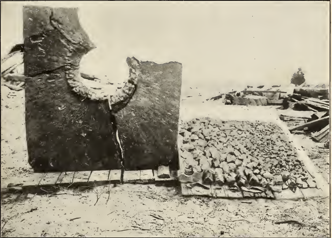
FIG. 6. SHOWING FRAGMENTS OF A \frac{5}{8} -INCH STEEL PLATE PUT BACK IN POSITION AFTER HAVING HAD A MAXIM SHELL EXPLODED IN IT. AT THE RIGHT ARE SHOWN SOME RECOVERED SMALLER FRAGMENTS OF THE PLATE.
