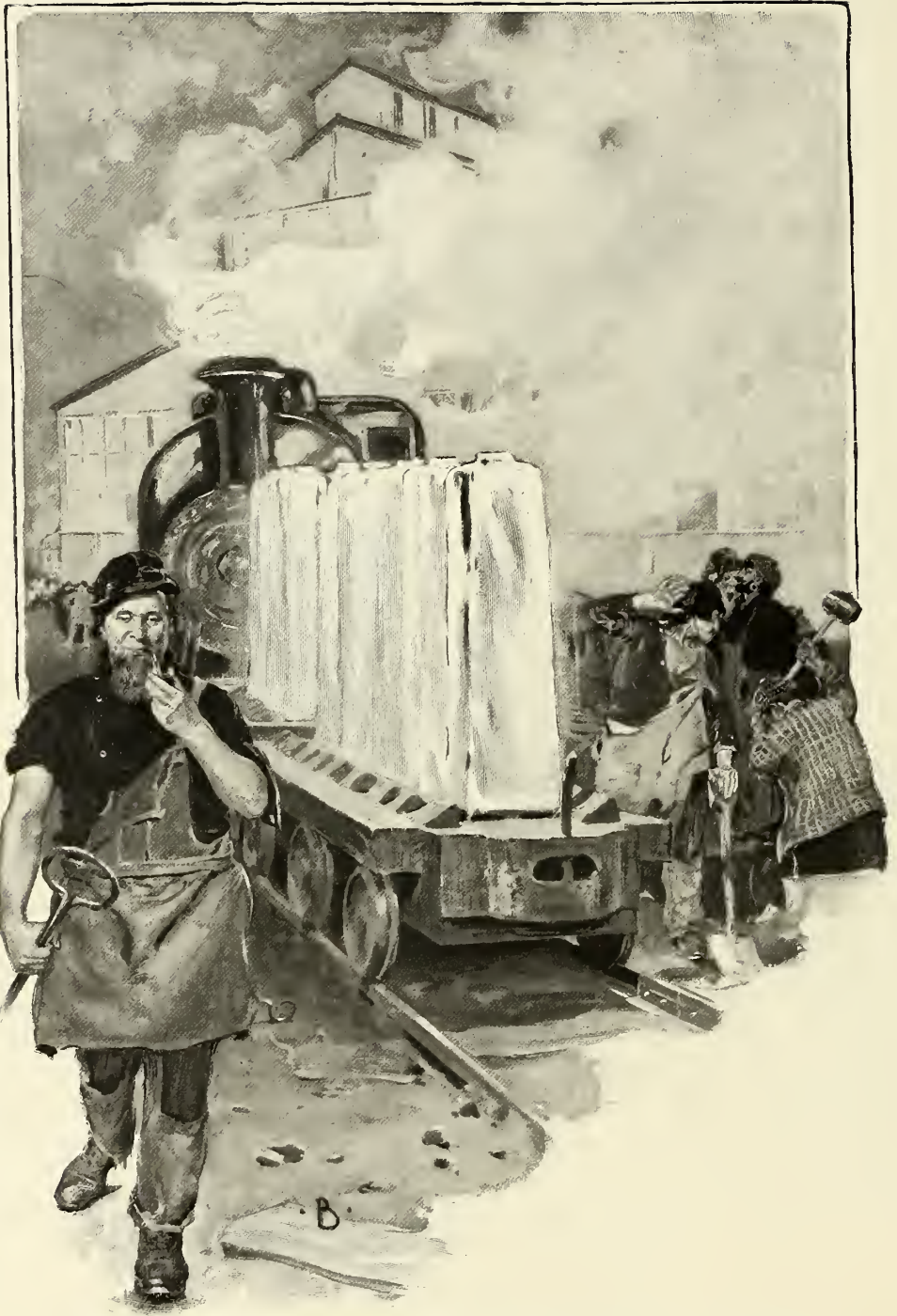
TRANSPORTING GLOWING STEEL INGOTS TO THE ROLLING-MILL. (SEE PAGE 442.)
