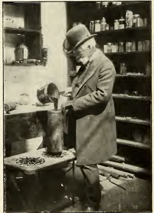
FIG. 9. FILLING A SHELL WITH MELTED MAXIMITE.
