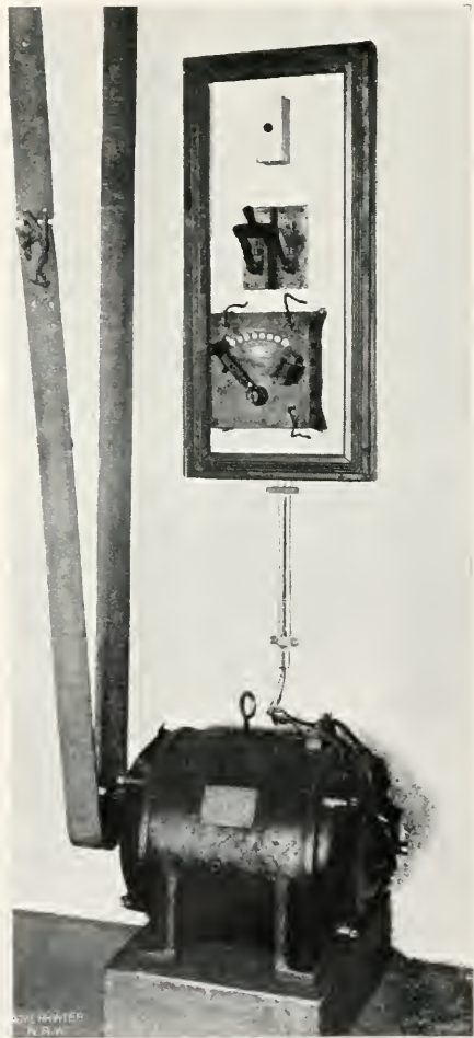
Electric Motor working various appliances in the Dairy, at the Hawkesbury Agricultural College, Richmond, N.S.W.
