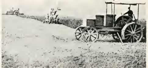
Plough worked to and fro in connection with two movable electric motors on a German farm. - Illustration by Siemens Bros., Ltd.
