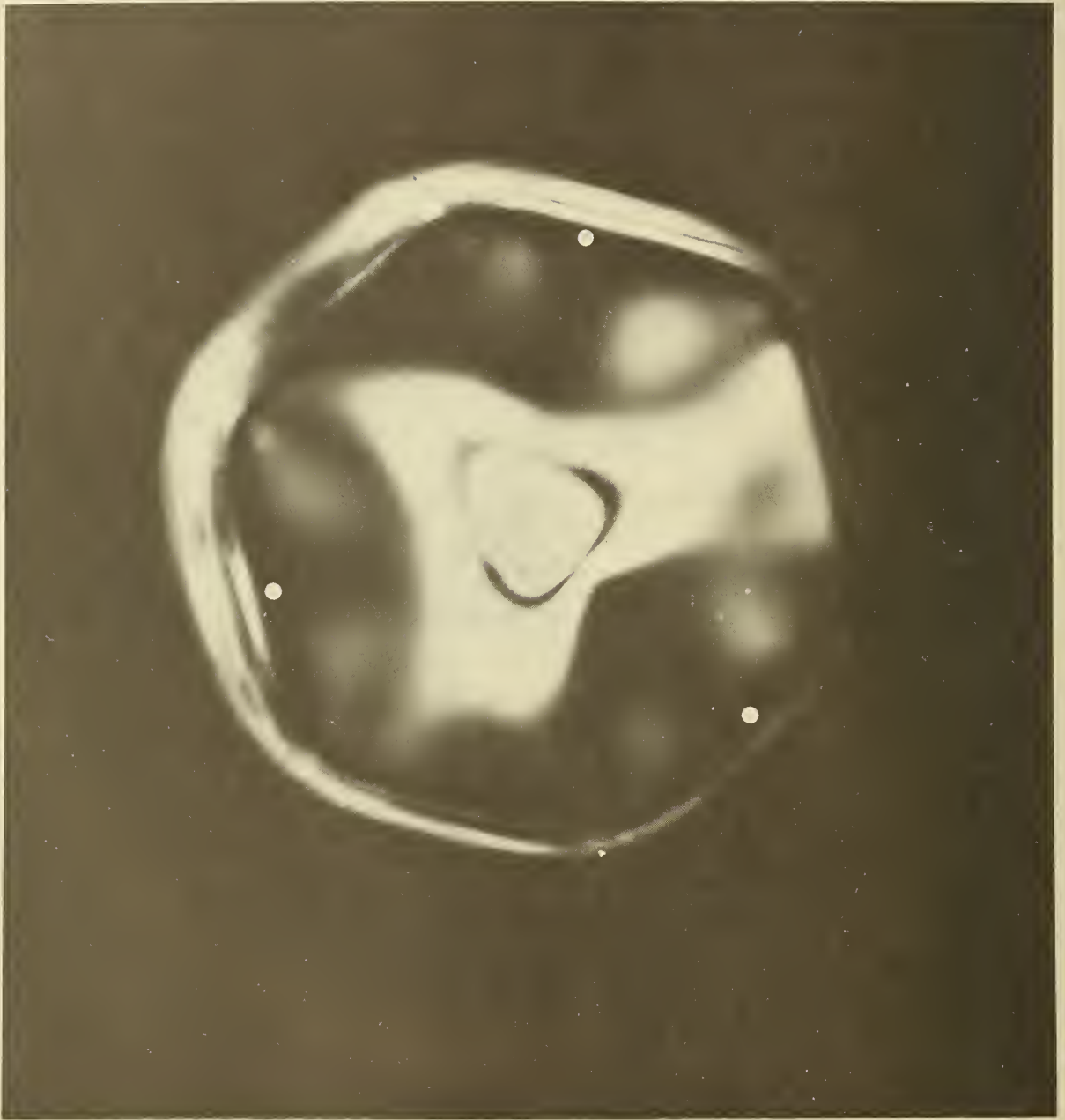
Figure 3. Birefringence pattern of the YAG boule place between circular polarizers.
