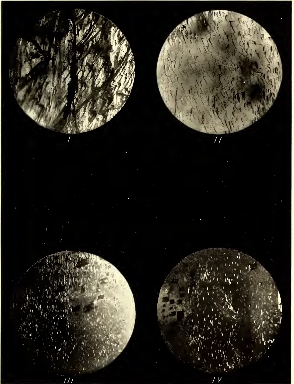
Natural etch figures on the Pala Spodumene. I. On the prism 1\bar{1}0 . II. On the prism 110 . III and IV. On the clinopinacoid 0\bar{1}0 .
