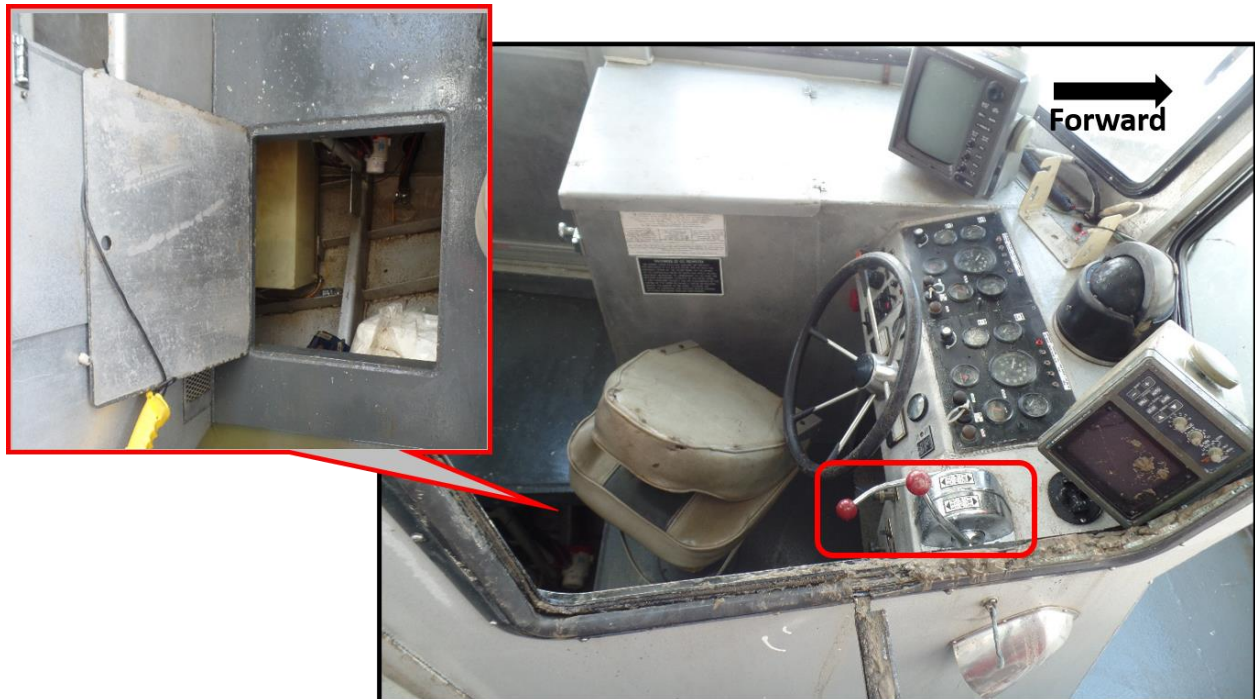
Cabin and control console of the MSRC 8-1 postaccident. The red rectangle indicates the position of the propulsion control levers at the time the vessel was recovered: full astern on the port engine and engaged astern on the starboard. The inset shows the crawl space below the cabin where the operator was later found, as viewed through the opened access cover directly behind the helm chair. (Source: Coast Guard)
