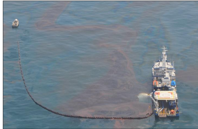
J-configuration deployment of oil spill boom by MSRC OSRV (right) and 32-foot workboat (left) during Deepwater Horizon oil spill response in May 2010. (Source: Munson Manufacturing, Inc)
