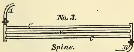
A. Feed Tube. B. Discharge Tube. C. Circulating Tubes.
