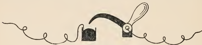
FIG. 9.—DIAGRAM OF MERCURY KEY.
