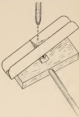
FIG. 73.—DIAGRAM OF TILTER. THE ROCKING MOVEMENTS ARE RECORDED EITHER BY ALLOWING THE ACCUMULATED FLUID TO ACTUATE A TAMBOUR, OR BY AN ELECTRO-MAGNETIC SIGNAL.
