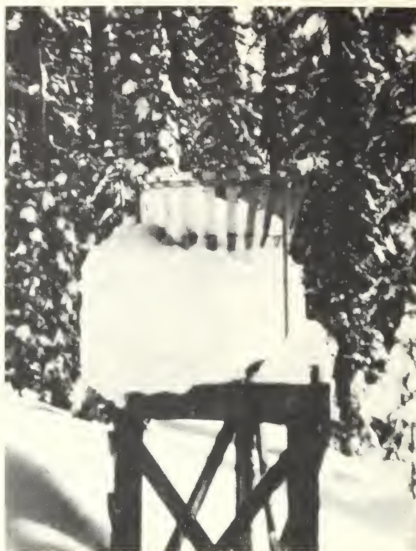
Figure 30. April 1, 1947. The Iron Creek gage at an elevation of 9,680 feet above sea level in the Fraser Experimental Forest, Colorado, is a Sacramento-type seasonal storage precipitation gage of 100-inch capacity. The water equivalent increment after November 16, 1946, was 11.25 inches, as compared with the water equivalent of a snow course based upon 10 samples surveyed in the vicinity of the gage of 11.75 inches.
