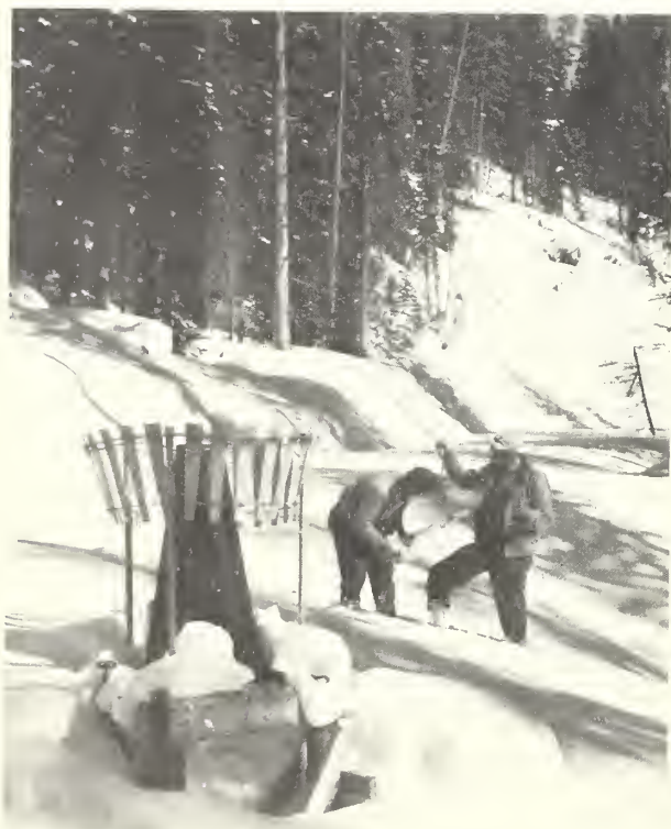
Figure 29. April 1, 1948. Snow survey being performed at the West St. Louis Creek seasonal storage precipitation gage, elevation 9,840 feet, in the Fraser Experimental Forest near Fraser, Colo. The water equivalent increment in the gage after September 25, 1947, amounted to 18.00 inches, as compared with 20.25 inches water equivalent as determined by a 10-sample snow survey being performed.
