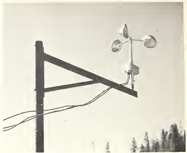
Figure 113. Low-level anemometer at windtower in the open. October 24, 1947.
