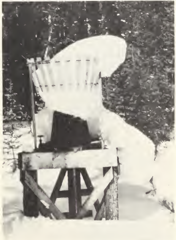
Figure 28. April 1, 1948. The East St Louis Creek gage, Fraser Experimental Forest, near Fraser, Colo. This is a 100-inch-capacity Sacramento-type seasonal storage precipitation gage installed at an elevation of 9,520 feet. The water equivalent gage increment after September 25, 1947, the date of servicing, amounted to 12.50 inches, as compared with 14.35 inches determined by a 10-sample snow survey in the vicinity of the gage.
