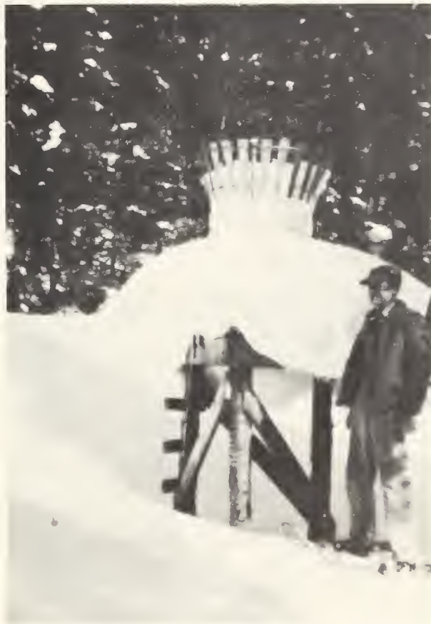
Figure 26. April 3, 1947. The St. Louis Pass gage at elevation 10,330 feet. This is a 200-inch-capacity Sacramento-type seasonal storage precipitation gage. The water equivalent gage increment after October 25, 1946, was 21.00 inches, as compared with the snow-water equivalent on the ground determined by 10 samples taken in the vicinity of the gage, of 23.11 inches. Note the blanket of snow on the platform and the cylinder of snow extending from the shield. It appears that the cylinder within and below the shield is formed by snow packing down from above as restrained by the shield and not by snow building up from the platform.
