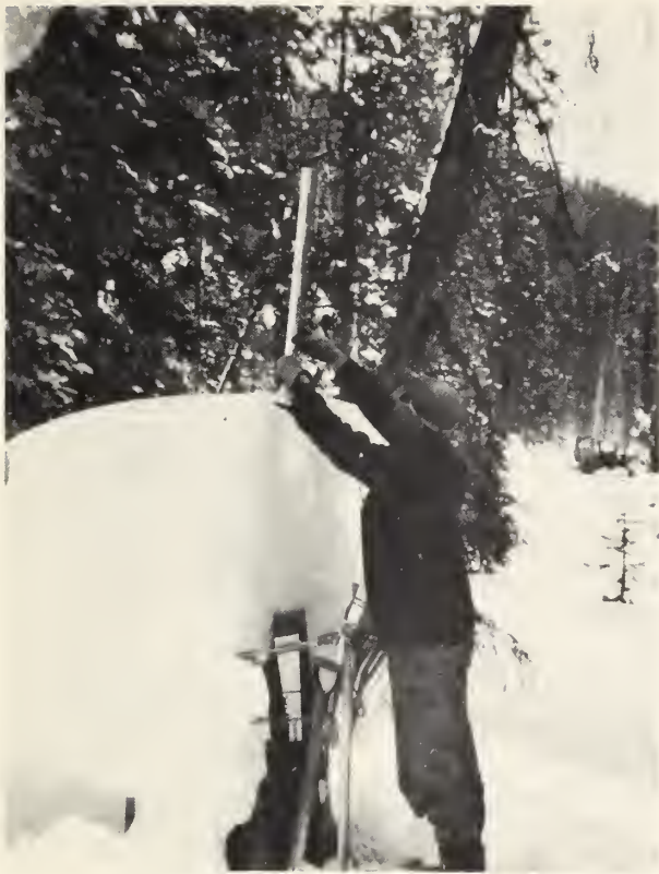
Figure 31. April 2, 1947. The West St. Louis Creek gage, an 100-inch-capacity Sacramento-type seasonal storage precipitation gage at 9,840 feet above sea level. The water equivalent gage increment after November 17, 1946, was 4.80 inches in the gage and 10.40 inches, including the snow samples in the mushroomlike top, as compared with a water equivalent of 28.77 inches as measured in a 10-sample snow course located in the immediate vicinity of the gage.
