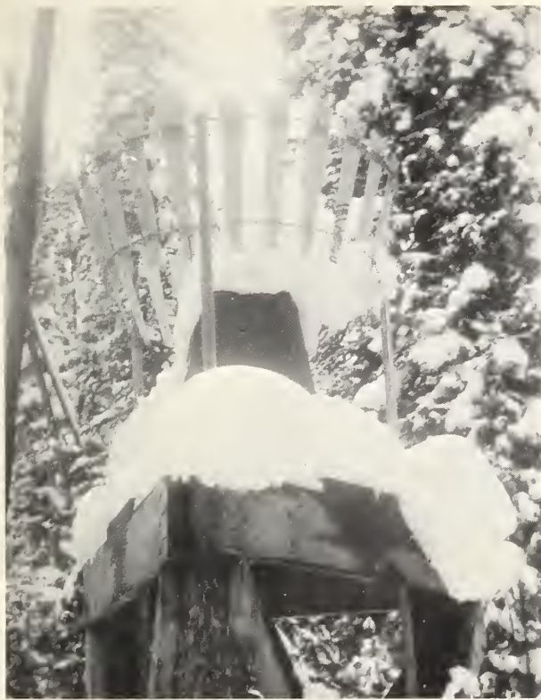
Figure 27. June 14, 1947. The East St. Louis Creek seasonal storage precipitation gage, 100-inch-capacity Sacramento-type, with Alter shield, as it appeared after the snowfall of June 14, 1947. The snow had a depth of 14 inches and a water equivalent of approximately 2 inches. This was sufficient to lodge in the space between the shield and the gage.
