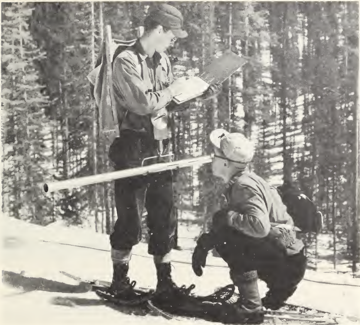
Figure 125. Weighing a snow tube and core of snow.
