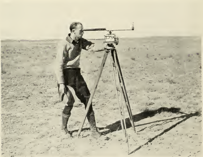
2. Observer stationed 3,000 feet from the tower with a recording telescope.
